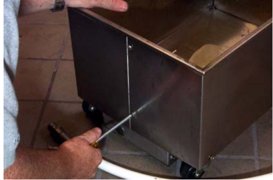
Remove screws securing outer panels.
